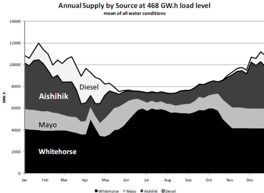
Figure 3: In this chart the energy supply includes Mayo B and the Aishihik 3<sup>rd</sup> turbine. Note that diesel-electric generation are required from November to June with the maximum requirements occurring in February to April, when wind energy is most abundant. Chart source from: YUB-YEC-1-37
